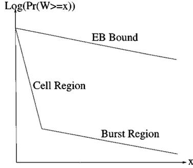
Fig. 1. Cell/burst regions, typical delay curve distribution, and EB bound.
