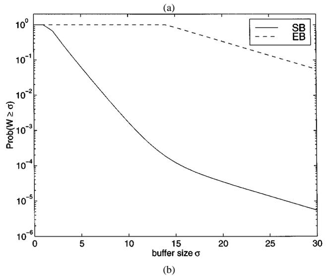
Fig. 2. (a) Bounding a distribution (exact) with a single exponential (EB) and with a sum of two exponentials (SB). (b) Bounds on the workload distribution of a multiplexer fed by two dependent processes: EB bound versus SB bound.
